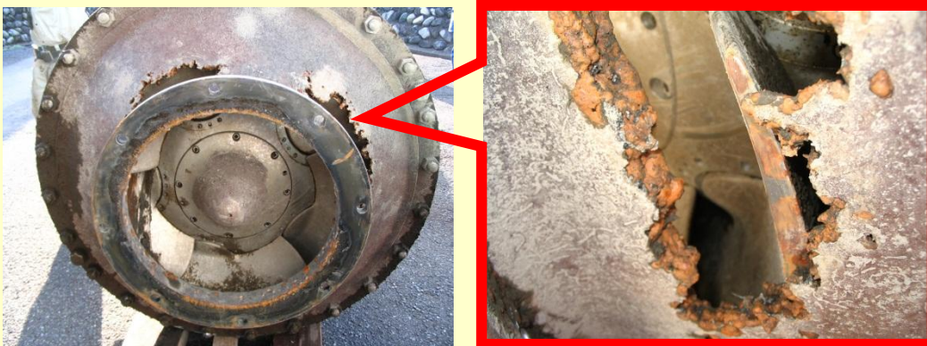
Case 1: Erosion by cavitation (holes on pump casing)
