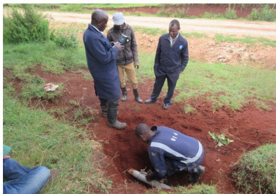
Verification of passing flow rate using UFM
