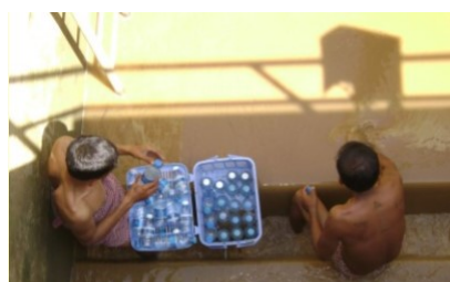
Sampling of backwash water at 1minute interval
